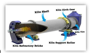
The rotary kiln is the central equipment where raw meal is heated and chemically transformed into clinker. This process occurs at high temperatures (~1450°C). To keep the kiln running efficiently and safely, several kiln spares (replacement parts) are used. These spares play crucial roles in rotation, heat containment, support, and sealing.
