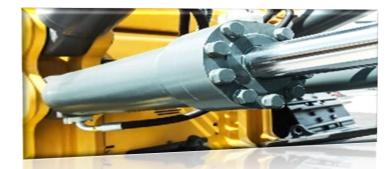
Hydraulic systems use pressurized oil to transmit power for high-force applications.
