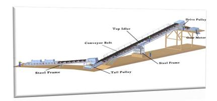
Conveyor systems are used extensively to transport materials like limestone, raw meal, clinker, gypsum, and cement between different processing areas. To keep these systems running efficiently, various spares (spare parts) are needed for maintenance, repair, and replacement.
